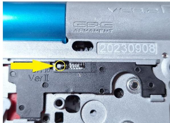
In replicas having gearbox other than V2 version, the cut-off lever will have a different shape, but will always be located somewhere near the bottom (or left side) of the sector gear and pushing it will similarly result with the closing of the sector gear switch, which ETU++ should detect and manifest.
